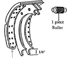
NOTE DISTINCTIVE "BENT-DOWN" TABS FOR ATTACHING RETAINER SPRINGS.
