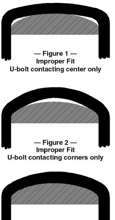
— Figure 3 — Proper Fit U-bolt is in uniform contact
