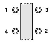
It is critical, when installing u-bolts to alternate from one leg to the other in criss cross fashion so that the torque is evenly applied to all four legs on each set of u-bolts. Tighten each nut only a small amount before switching to the leg diagonally across. Continue alternating until all four legs on each set reach the specified torque.
