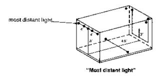
Determine: Wire size required for the clearance light circuit having eleven lights with No. 97 bulbs
